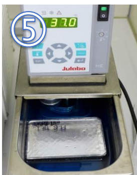
Thawing of the free floating assay for only 1 min in the water bath
