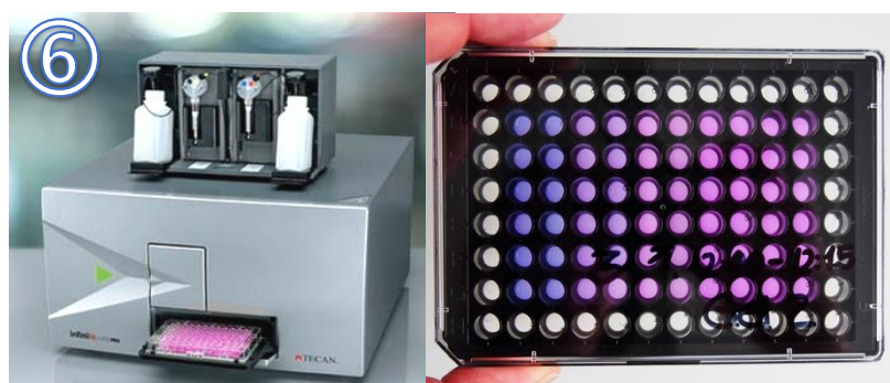
Automated application and photometric evaluation of the in vitro toxicity test for 4 different drug concentrations by use of a plate reader with reagent injector (pipette - incubate - read)
