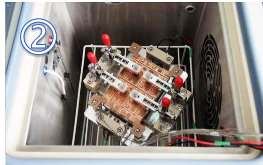
Vital cryopreservation of the multiwell assay in a LN 2 convection freezer by use of our multiwell RACK
